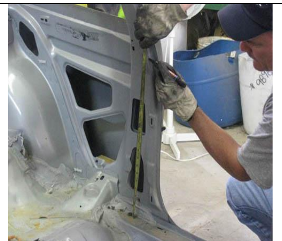
Main Loop Height Bottom Mounting to B-Pillar
