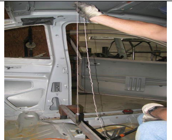
Main Loop Height Bottom Mounting to Roof
