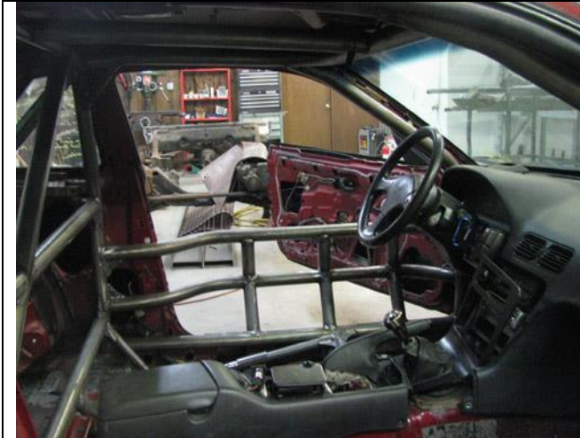
Nascar Door Bar made to fit around B-Pillar
