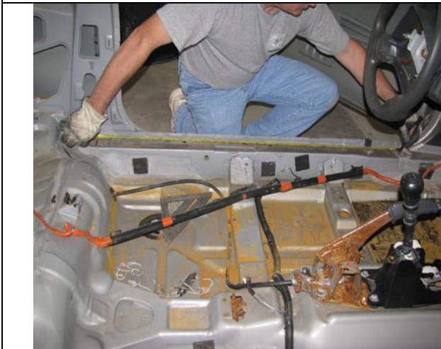
Bottom Door Bar Length Measure Main Loop Mark to Windshield Post Mark For Angled Door Bar Measure From B-Pillar to Roof Length Line to Windshield Post Mark Used for a X Design or Drag Design
