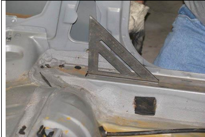
Main Loop Location Mark Note should be used as back side of main loop
